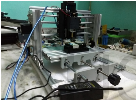
Photograph 2: Final CNC Machine..
